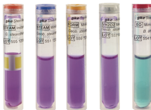
Fig. 2: Instant-Mini-Bio-Plus SCBI for steam, standard SCBI for steam, formaldehyde, hydrogen peroxide (glass fiber carrier) and ethylene oxide sterilization processes.
